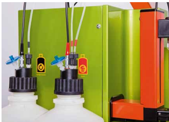
Figure 2.5: Connect the according color-coded tubing and sensor cables to the appropriate connectors on the waste bottle closure and the Storage Solution bottle closure.
