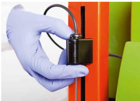
Figure 5.4: Lower the robotic needle arm holder by another 5 mm.
