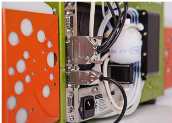
Figure 2.8: Connect the cable of the 2D code reader to the RS232/BCR port of the MACSQuant Instrument.
