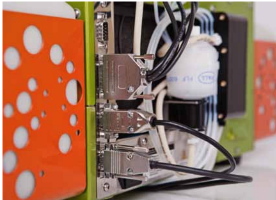
Figure 2.15: The MACS MiniSampler cable is attached to External CAN port.
