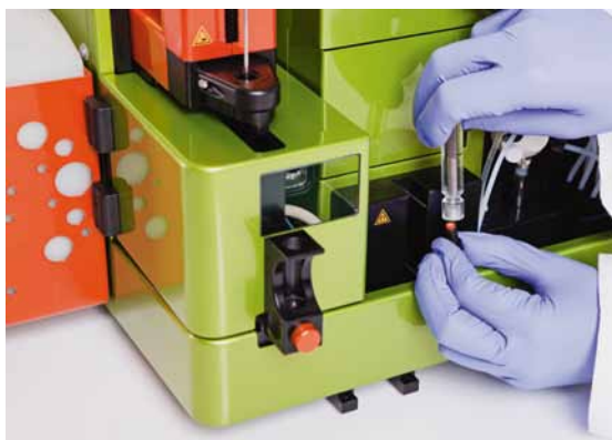
Figure 2.20: Installation of the bottom connector to the MACSQuant Column.
