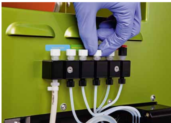
Figure 2.4: Connect the color-coded tubing to the according position of the bottle distribution block.
