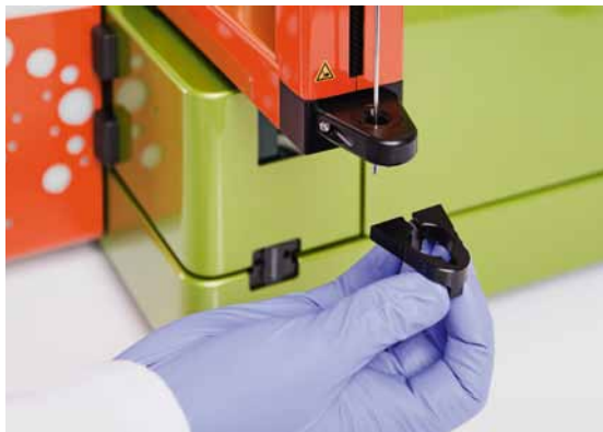
Figure 2.10: The needle guard is attached to the robotic needle arm in order to protect against the risk of puncturing bodily parts.
