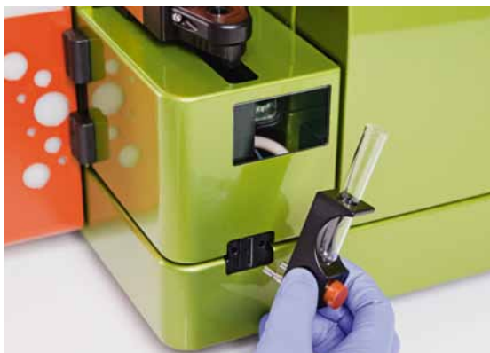
Figure 2.11: Install or remove the Single Tube Rack by simply plugging or unplugging.
