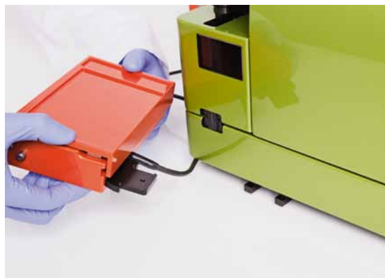
Figure 2.12: MACS MiniSampler slot at the front of the MACSQuant Instrument and the corresponding guiding on the MACS MiniSampler.
