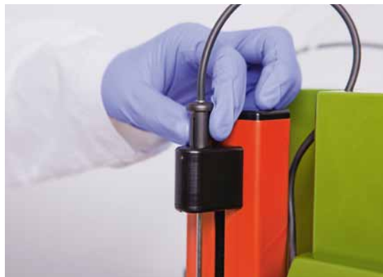
Figure 2.3: The uptake needle is placed into its guiding at the robotic needle arm.
