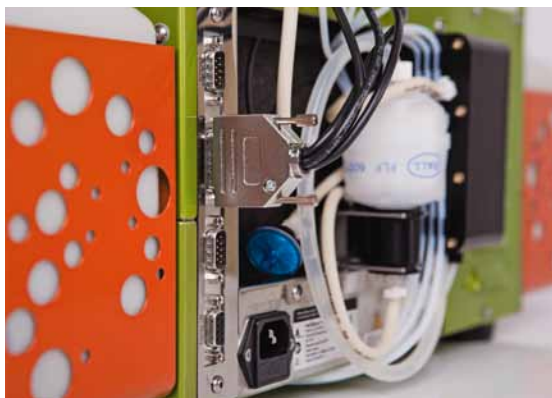
Figure 2.7: Connect the sensor cables to the sensor cable port on the back of the MACSQuant Instrument.
