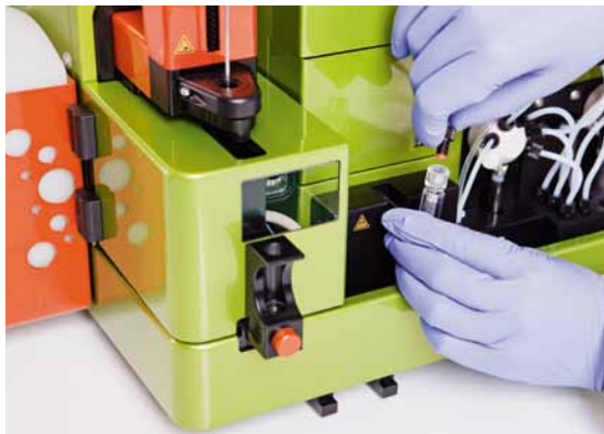
Figure 2.21: Installation of the top connector to the MACSQuant Column.
