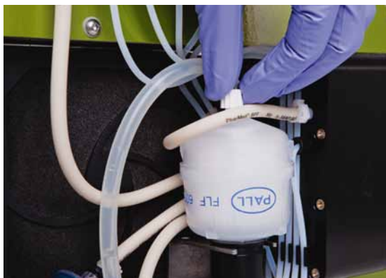
Figure 2.9: Purge the system by opening the white lid on top of the sheath particle filter.
