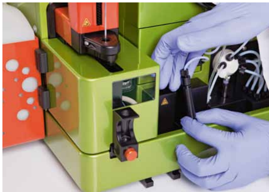
Figure 2.19: Removing the column substitute from the MACS Enrichment Unit.
