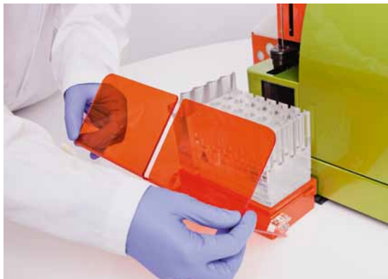
Figure 2.18: The protective cover is installed on the MACS MiniSampler.
