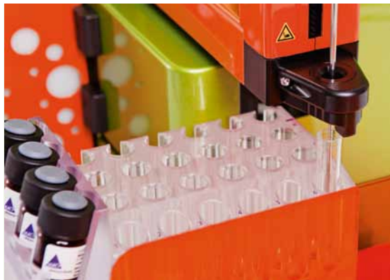
Figure 5.8: Calibration of the Chill 5 Rack by defining the position D6.
