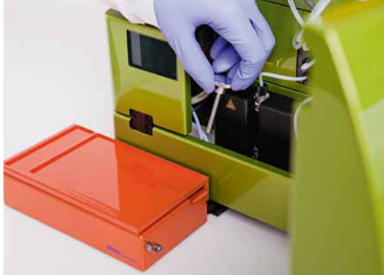
Figure 2.14: Fixing the MACS MiniSampler with the according screw.
