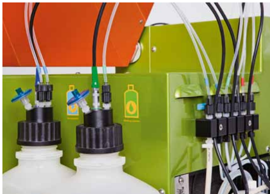
Figure 2.6: Connect the according color-coded tubing and sensor cables to the appropriate connectors on the Running Buffer bottle closure and the Washing Solution bottle closure.
