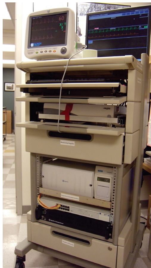
This self-contained and portable telemetry system is used for alarm training at Boston Medical Center's Solomont Clinical Simulation and Nursing Education Center.
